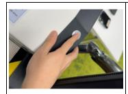
◀ If the **Touchscreen** ③ is black and the blue power light is flashing, press the **Power Button** ⑤ once to wake the scanner from standby mode. The power button will illuminate solid blue, and a **Warming up** window will appear on the touchscreen. Once the scanner is ready, tap **Ok** to continue.
