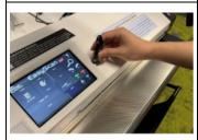
■ Insert a FAT32 or NTFSformatted USB drive into the USB Connection Socket ② to prepare for saving the scanned file.
